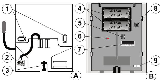
Figure 1: A - base; B1 - front part of the case with electronics; 1 - mounting holes; 2 - external sensor JB-TS-PT1000 wire terminal; 3 - cover lock screw; 4 - battery holder; 5 - external antenna AN-868 connector; 6 - light signalization; 7 - production number; 8 - discharging button; 9 - wire terminal connector
