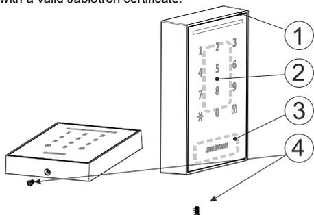
Fig. 1: 1 – system indicator, 2 – reading zone 125 kHz, 3 – reading zone 13,56 MHz, 4 – locking screw
