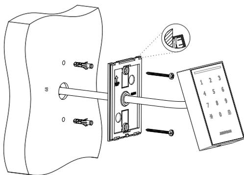
Fig. 2: Keypad installation
